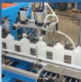
Integrated leak test station with bottle blow off option
