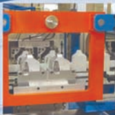
Wide punch platen allows single or multiple nest/die set ups; keyed backplate allows quick nest/die changes
