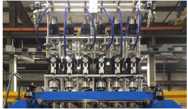
6-head with parison programmer and top finish
